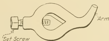
Fig. 188—A lathe dog of standard type
